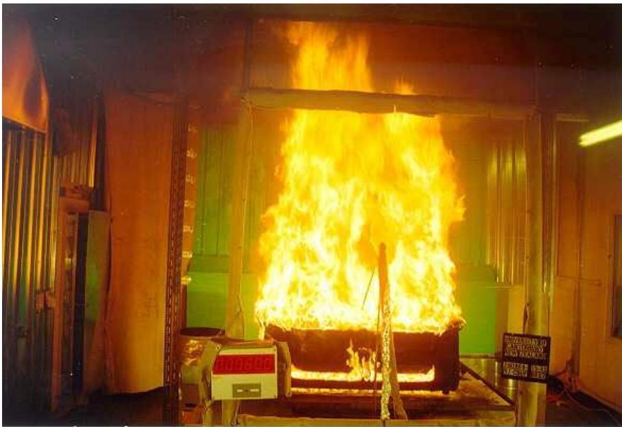
Figure 15: UC Furniture Calorimeter during NZ-CBUF test. A two-seat furniture item at a peak HRR of \sim 2250 kW, approximately 180s from ignition
